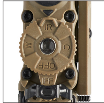
Rotary mode selector switch & IFF beacon
