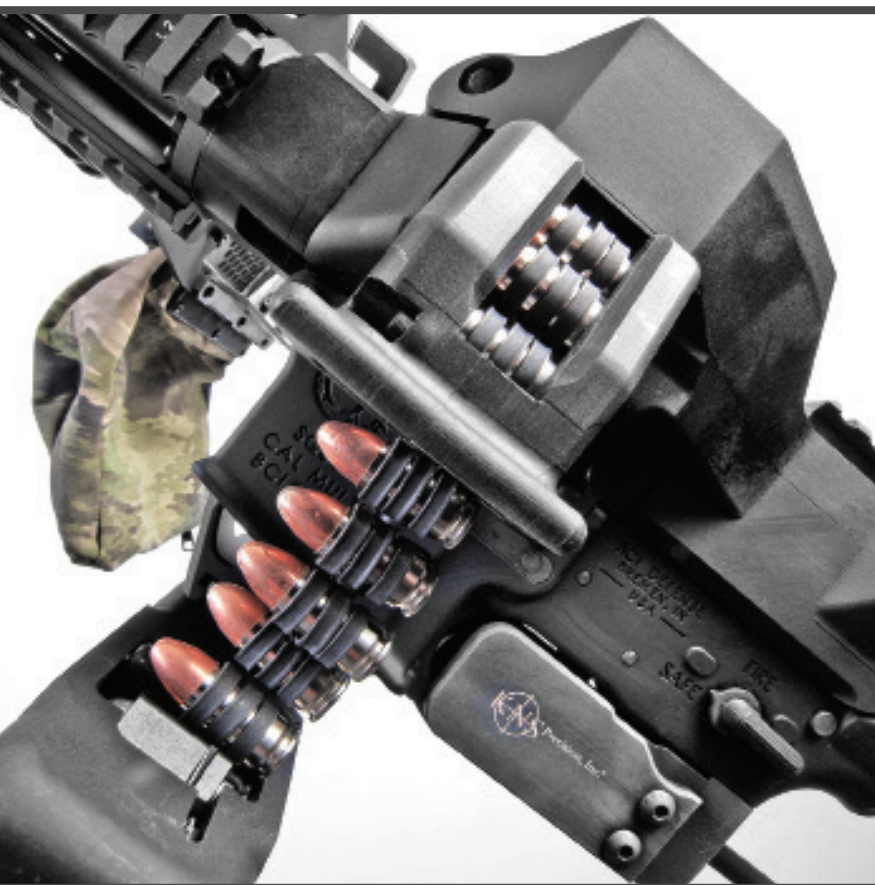
The disintegrating-link belt feeds from the left side of the receiver (left). Adding the KNS Gen 2 Spade Grip and Firestorm Works Tripod (below) makes the FM-9 resemble a heavy machine gun.
