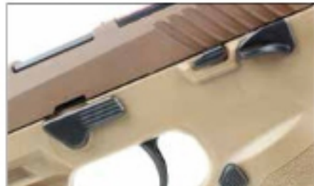
Operator controls: the M17 slide release is surprisingly small but most shooters "slingshot" the slide to release it.
