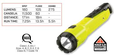
The Dualie Rechargeable's bright light shines both ahead of you and downward to help avoid slips, trips and falls. A magnetic clip features a hang hook for hands-free use. Save on battery costs - it's rechargeable! Intrinsically Safe - Class I & II, Div.1. IP67-rated; dust-tight and waterproof to 1m for 30 minutes; 2m impact resistance tested.
