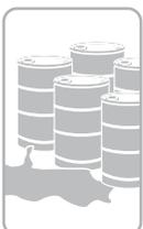
**DIVISION 2** locations are where ignitable concentrations are not likely to exist under normal operating conditions or where Class 3 materials are stored or handled.
