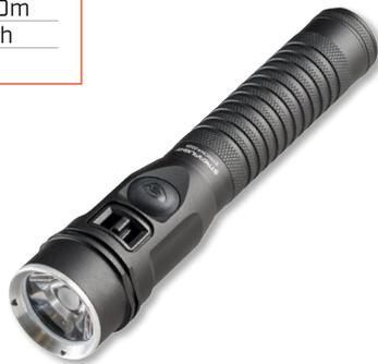
The Strion 2020 features independently functioning head and tail switches along with an intuitive mode selector switch for ease of use. Select high for brightest light or low for extended run time. Long-lasting lithium-ion rechargeable battery offers multiple charging options using existing Strion smart chargers and bank chargers. IPX7-rated; waterproof to 1m. Corrosion-resistant sealed glass lens.
