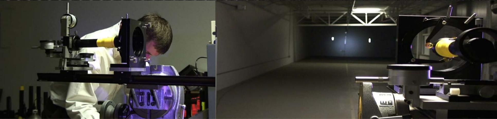
**Purpose:** To provide a procedure to determine the peak beam intensity, reported in units of candela, of the device's beam within 30 seconds to 2 minutes of operation.
