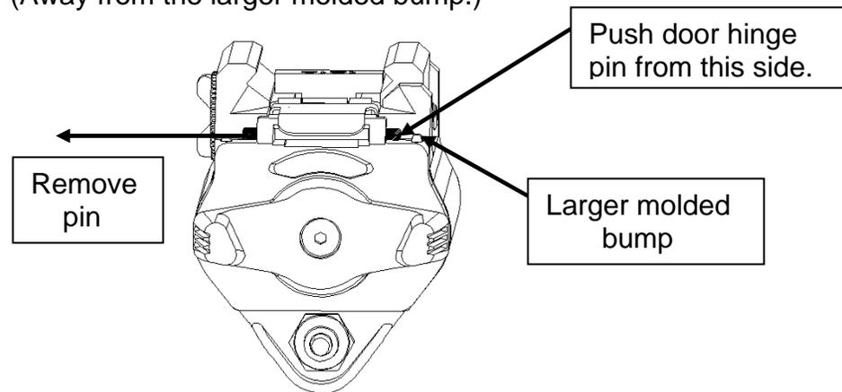
When enough of the door hinge pin becomes exposed it can be removed by grasping it with the pliers (slightly lift the pin upwards to clear the smaller molded bump) and sliding it free.
